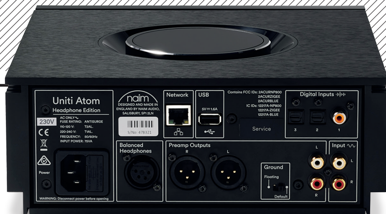
ABOVE: Alongside wireless [inside] and wired Ethernet ports are USB-A, coax, two Toslink optical and one pair of analogue inputs (RCAs). Preamp outs are offered on RCAs and balanced via 3-pin XLRs, with a balanced headphone output on a 4-pin XLR
