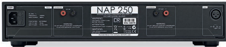
ABOVE: Input is via a single 3-pin XLR with pin 1 assigned to the left channel, pin 2 to the right and pin 3 as common ground. Speaker outlets are simple 4mm sockets
