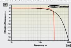
ABOVE: Extended high frequency response at 10W/80hm [black] vs. typical resp. of Naim's DACs [red]
