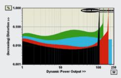
ABOVE: Dynamic power output versus distortion into 80hm (black trace), 40hm (red), 20hm (blue) and 10hm (green) speaker loads. Max. current is 8.4A
