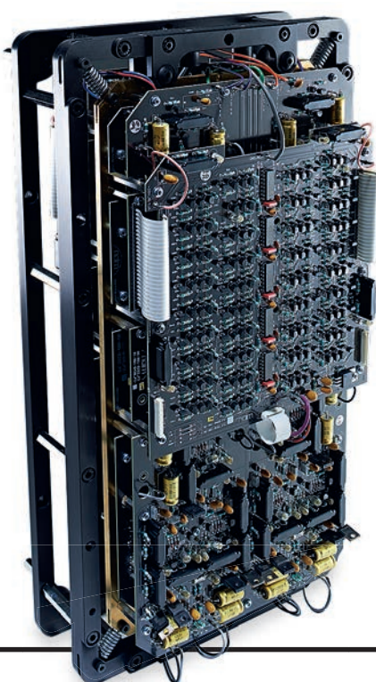
RIGHT: The power supply, control and audio stages of the NAC (left) and NAP S1 (right) are suspended on CNC-machined frames, creating circuit 'floors' within the massive chassis
